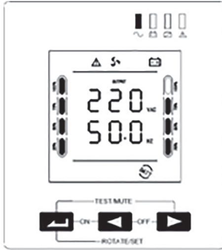
Figure 12. Display of the UPS
