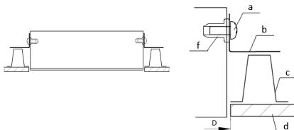
3. Remove the grill from unpacked luminaire, put mains cable through the hole in luminaire's body.
