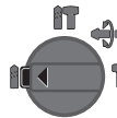
Position for drilling without impact in wood, metal, ceramic and plastic as well as for screwdriving
