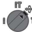
Vario-Lock position for adjustment of the chiselling position. The mode selector switch does not latch in this position.
